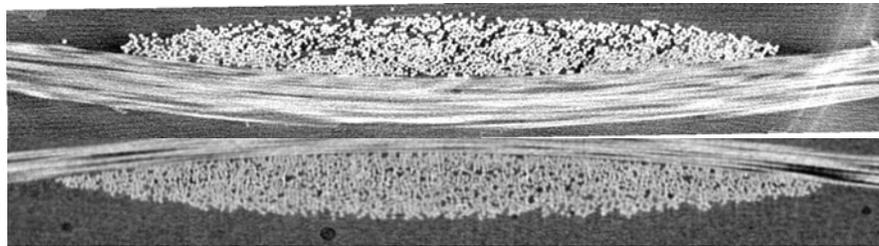
Fig. 2 Tomography reconstructed slices of a glass plain weave. Undeformed state (top) and biaxial tensioned state (bottom) - different scales.
