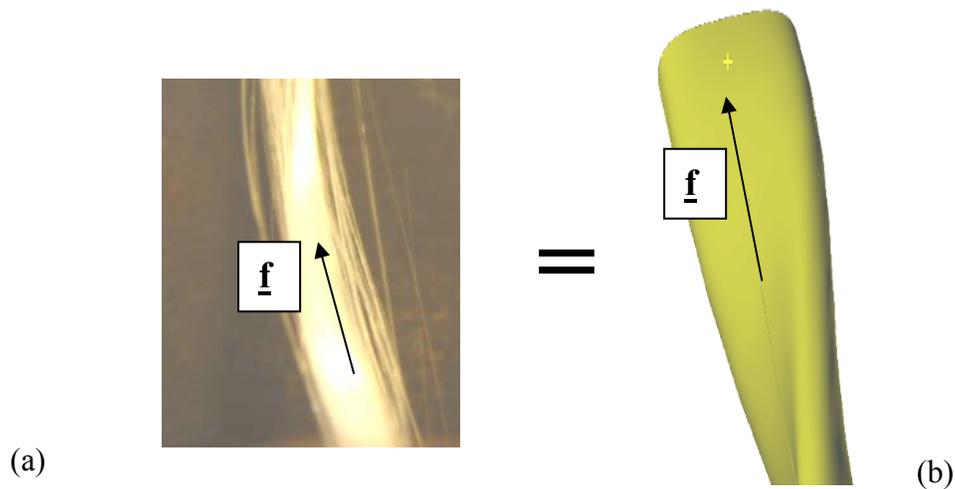
Fig. 1. Fibre direction  $\underline{\mathbf{f}}_1$  inside a yarn. (a) actual yarn (b) equivalent continuum model.
