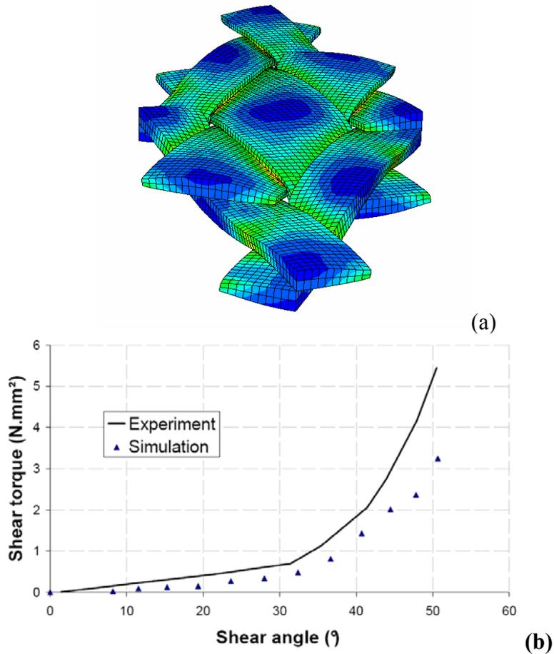
Fig. 3 (a) Deformed unit cell with contours of local compaction;
